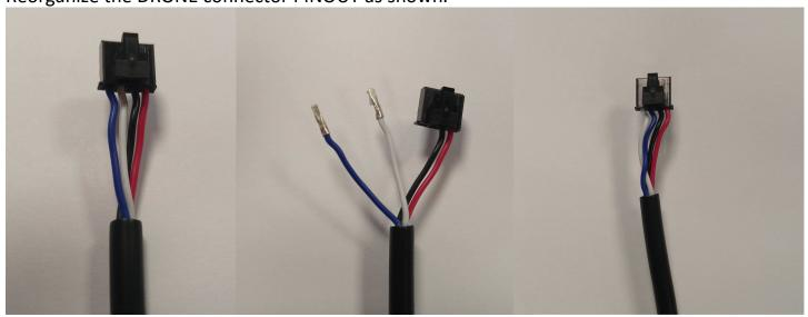
Connect the DRONE in the EVO-ONE **BLUE** Connector with clip as shown.
